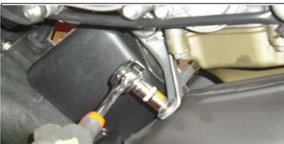
**ENG** Unscrew the nuts of the front bracket support silencer left and right
