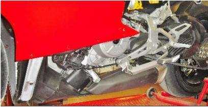
**ENG** Remove the lower fairing right and left of the bike, removing the screws
