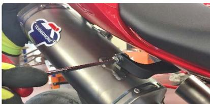
**ENG** Insert right silencer (7) and screw it to the silencers support bracket (18) through the screw (12) and washer (25) supplied.
