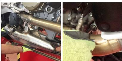
**ENG** Remove the pre-silencer. Remove the screw and bottom pre-silencer support bracket
