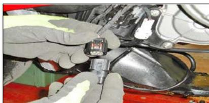
**ENG** Disconnect the valve and insert the connector protective cap, in the pack
