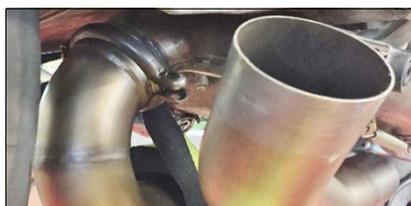
**ENG** Fix the central body to the original collector using the original clamp, screw and nut and tighten
